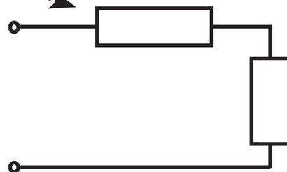
IMPEDANCE (PARALLEL) displays the impedance seen from the test port. The impedance is resolved into the real (resistive) part and imaginary (reactive) part connected in parallel. The corresponding inductance or capacitance is also displayed according to the sign of the reactance.
