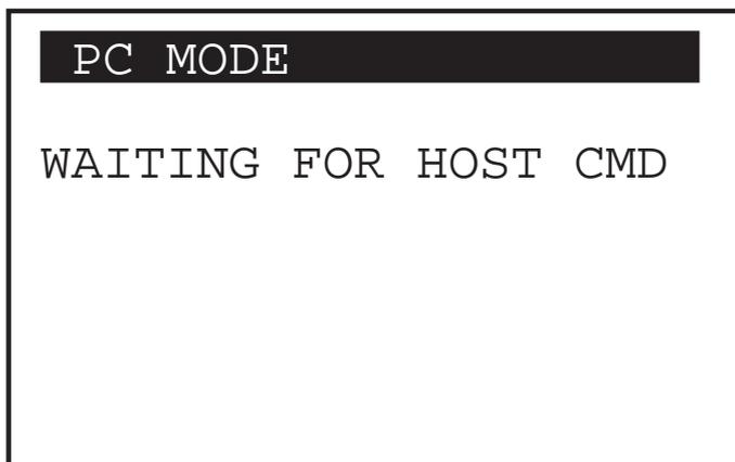
To command T100 to tune to a specific frequency, the host program shall transmit a six-digit frequency in ASCII characters via the serial port.
