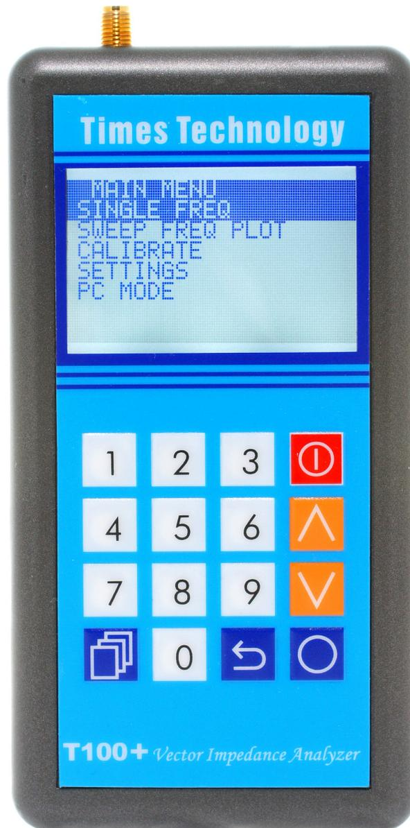
T100+ is a state of the art portable Vector Impedance Analyzer. This powerful yet handy instrument is specifically designed for the advanced amateur radio experimenters working at the VHF and UHF bands.
