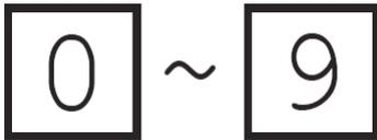
**NUMERICS** : Use these keys to enter the desired frequency directly. Frequencies within the valid operating range will automatically be aligned to the 25KHz steps. Frequencies outside the valid operating range will be ignored.
